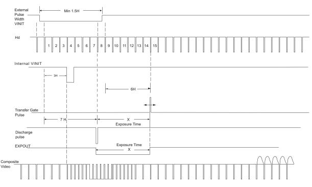
For the progressive format, one frame of video output will start from the rising edge of the pulse width control. At async mode with external pulse input high, the video output will be disabled as the camera continues discharging the CCD image, providing black video only.
